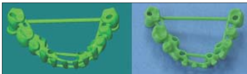
Screen shot of a virtual design pattern (left) and the actual wax-jet pattern before casting (right). Photo courtesy of Dr. Stephen Schmitt
